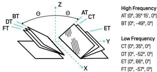
Figure 3. Singly-Rotated Zero Temperature-Coefficient Resonators
