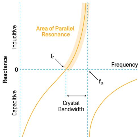
Figure 8. Crystal impedance - series vs parallel resonance
