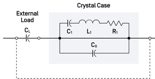
Figure 7. Simplified Equivalent Circuit
