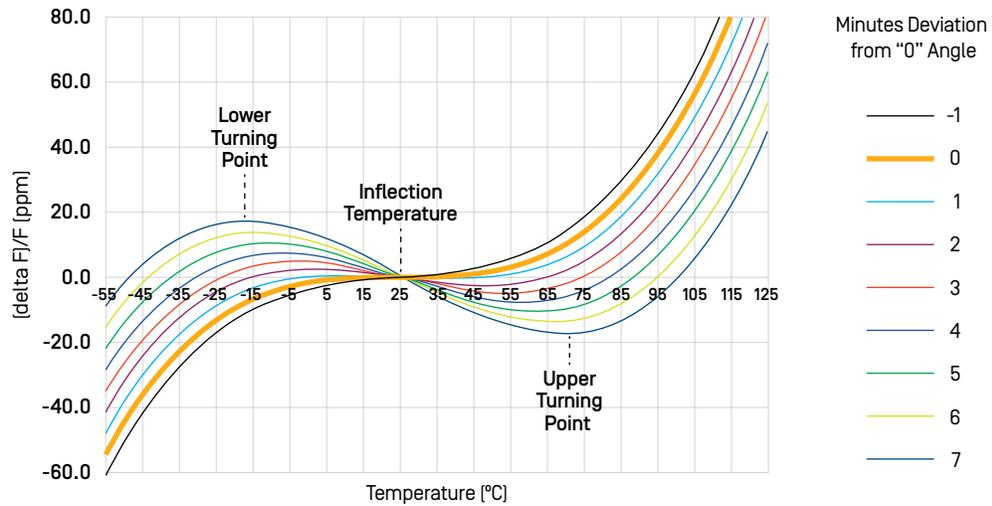
Figure 2. AT-cut Frequency vs. Temperature Curves
