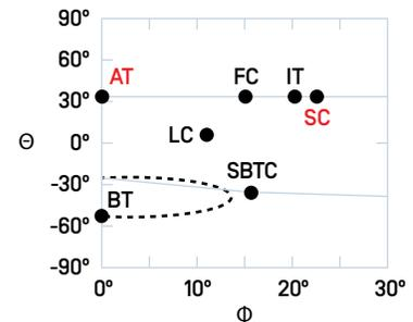
Figure 5. Various degrees of freedom-from-stress bias for doubly-rotated orientations that have zero temperature-coefficients
