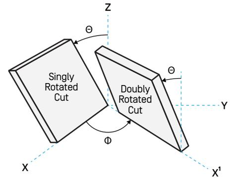
Figure 4. Singly- and Doubly-Rotated Crystal Cuts
