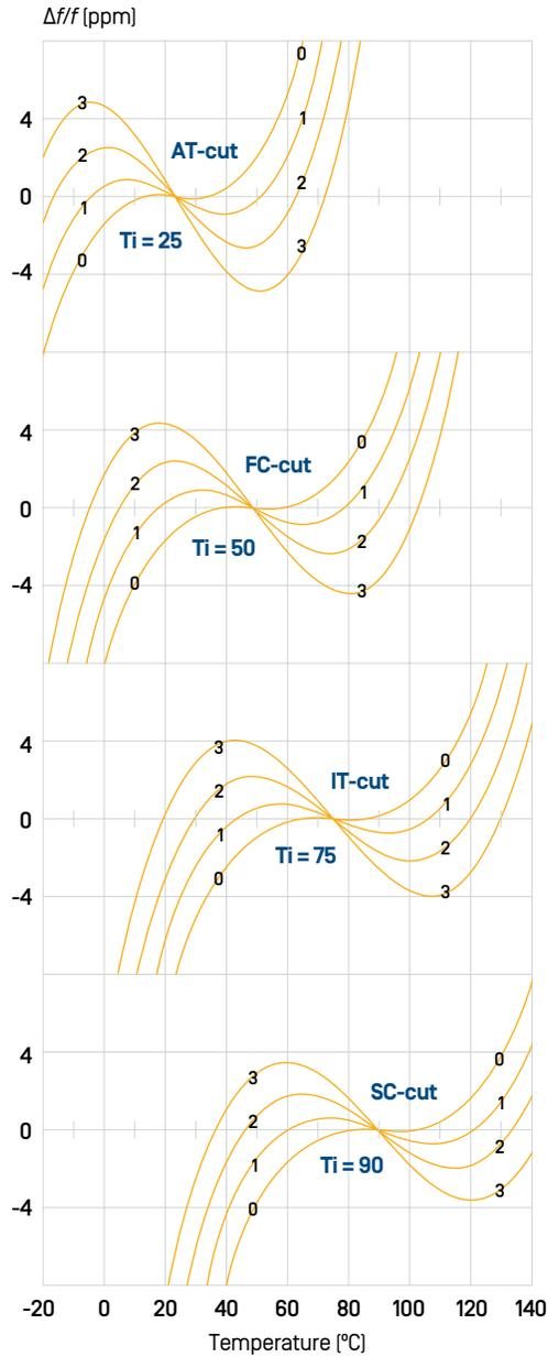
Figure 6. Generalized F-T curves for standard crystal cuts illustrating typical inflection temperatures
